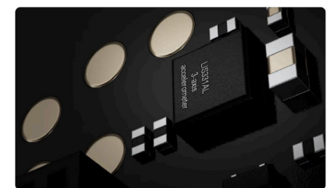
Built-in accelerometer: reports dismantling and impacts
