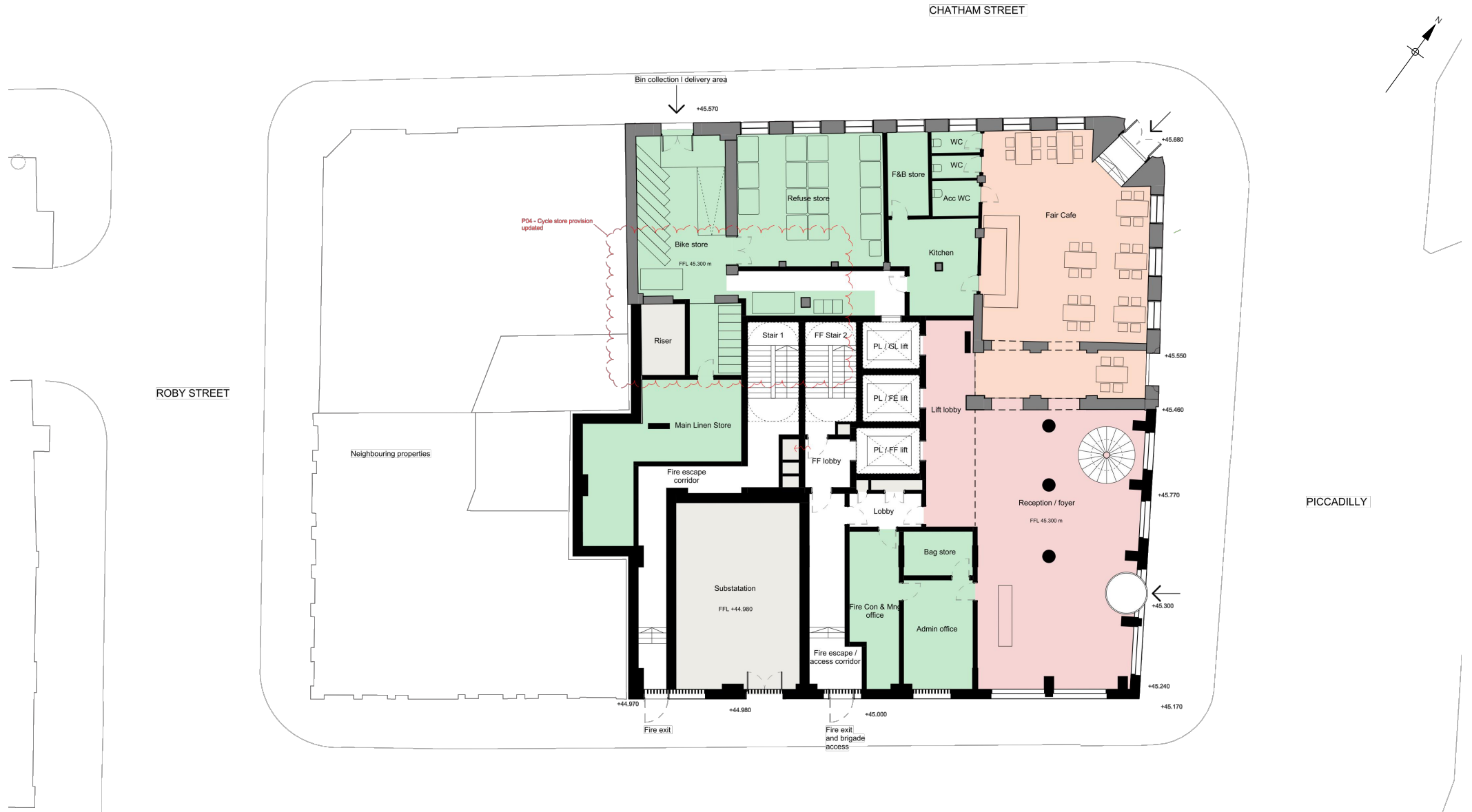
Figure 4 Plan of the Proposed Ground Floor 1:250 at A4
