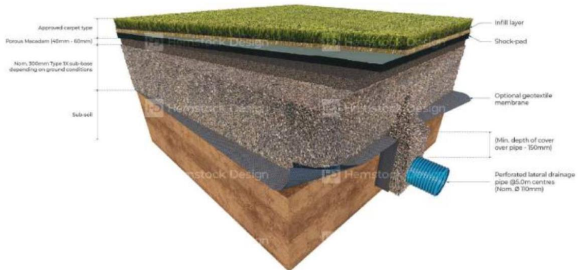
Figure 8 – Typical Synthetic Turf Pitch Surface Drainage
