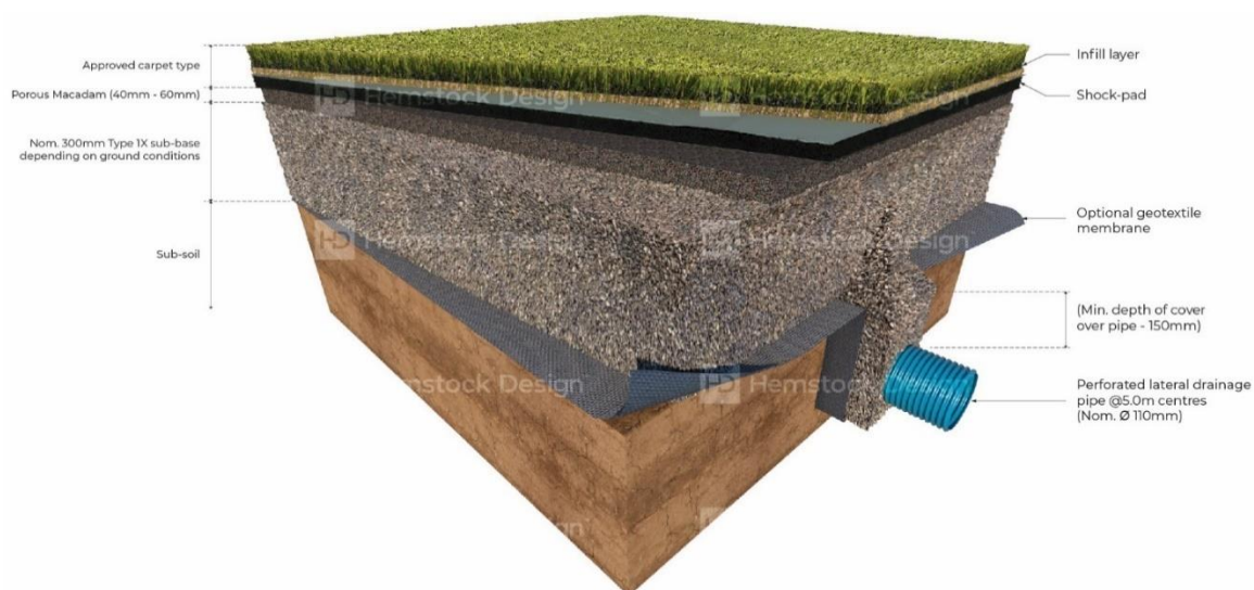
Fig. 8 - Illustrative profile of the new MUGA AGP, with sand infill needle-punch carpet over a shock pad and porous bitmac layer, drainage layer aids attenuation of peak flows.
