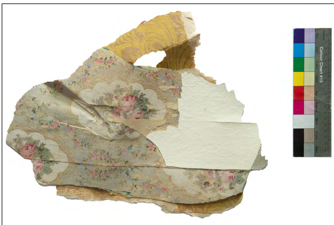
Appendix 2.71: GII Detail of wallpaper sample recovered from chimney breast, north wall (obverse) (D196) (Scale 20cm)
