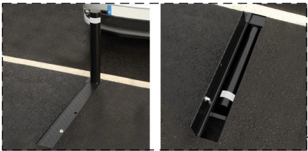
2no. Broxap BX015550 or similar countersunk foldable bollards in front of gates. Zinc plated and polyester powder coated in black. Reflected strip only if required. To be raised as default and lowered by concierge when necessary.
