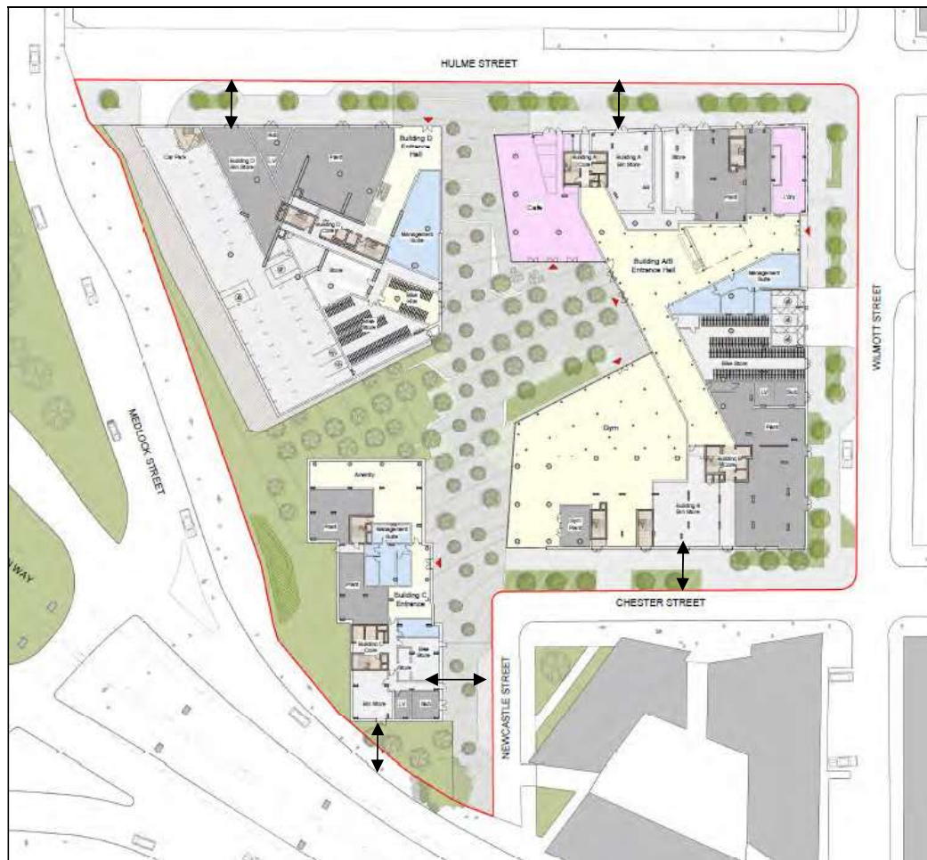
Figure 4.2: External Waste Routes
