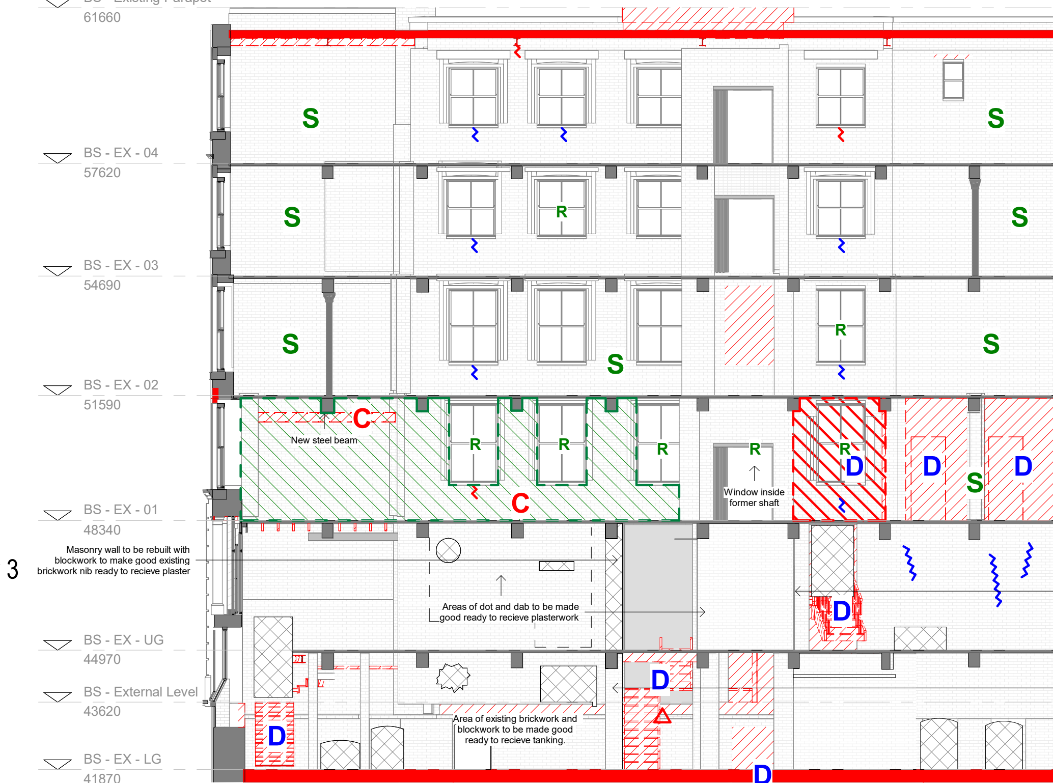
D | D - INTERNAL ELEVATION - PERIMETER WALL. 1: 100
