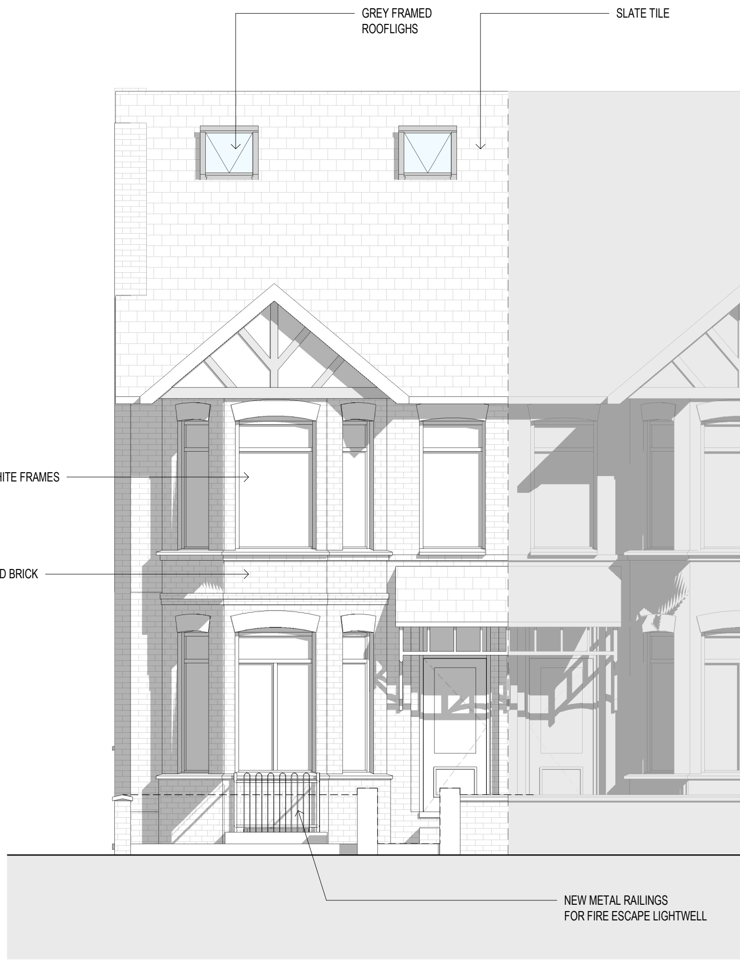
01 PROPOSED ELEVATIONS - NORTH-WEST
