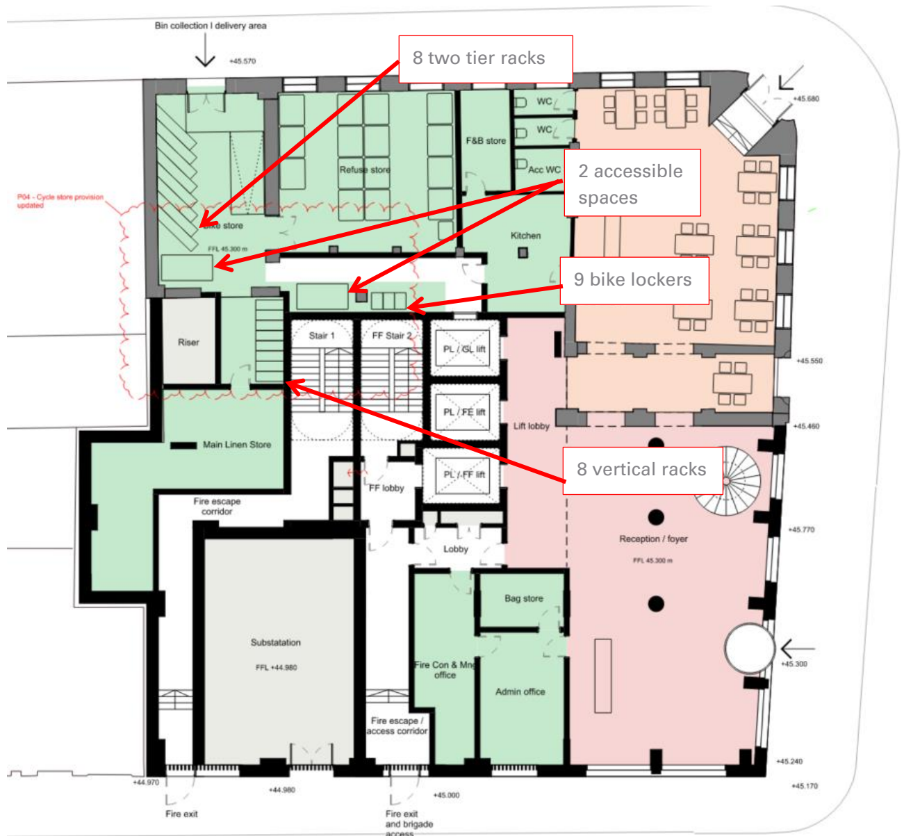
Figure 3.3: Proposed Ground Floor Layout. (Extract from Bennetts Associates Drawing No. HMP-BA-20-L00-DP-A-0)
