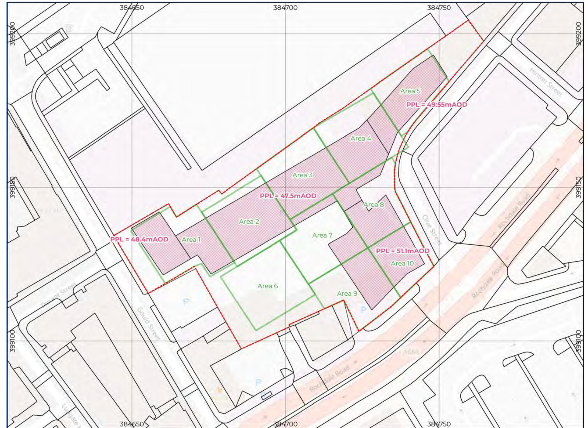
Figure 5 – Piling Platforms and Earthworks Areas
