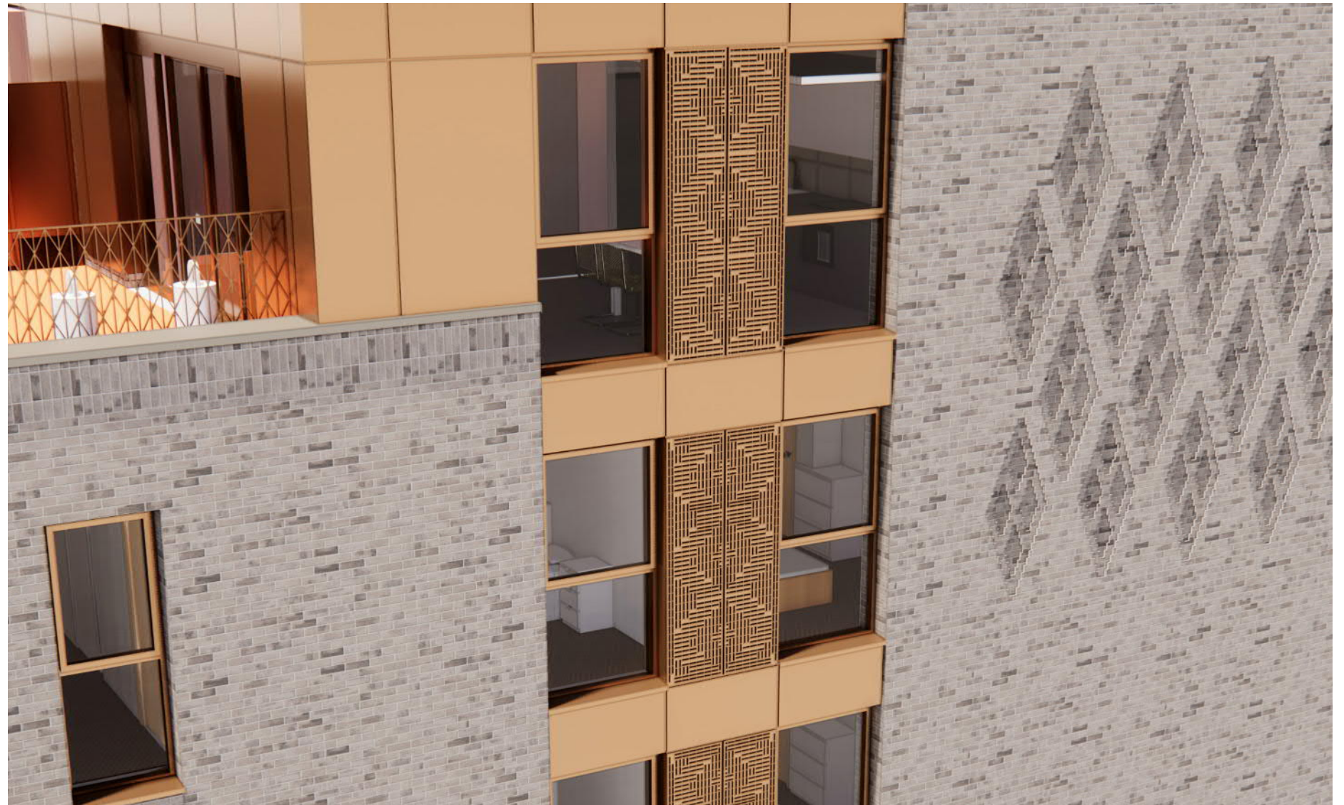
Perforated Panel - 20mm Joint
