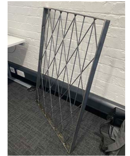
Images above of the fabricated prototype for the Juliette balcony (unpainted).
