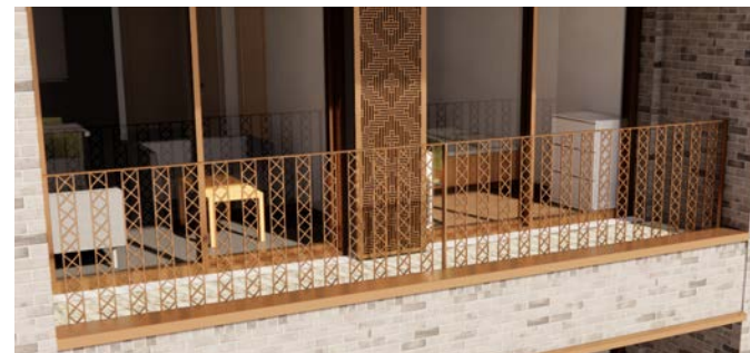
Option 05 Pros - closely aligns with 'textile' motif pattern, bespoke and decorative. Cons - not enough visual permeability, pattern too distracting, introduces a new linear language.
