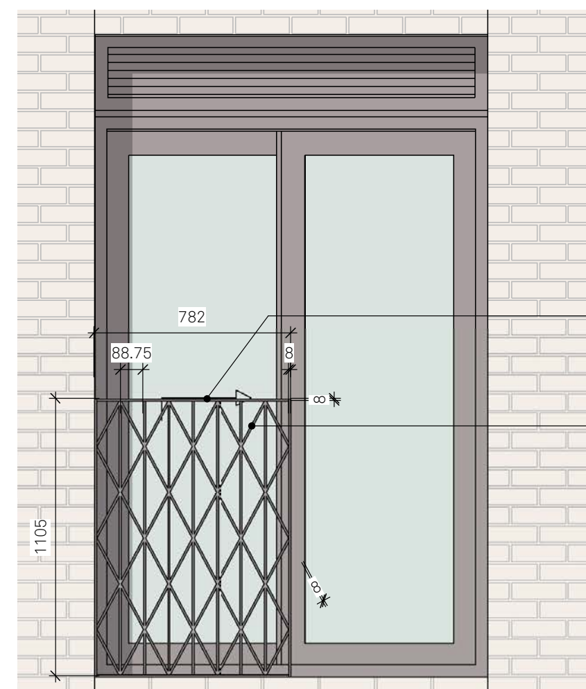
Option 05 Pros - closely aligns with 'textile' motif pattern, bespoke and decorative. Cons - not enough visual permeability, pattern too distracting, introduces a new linear language.
