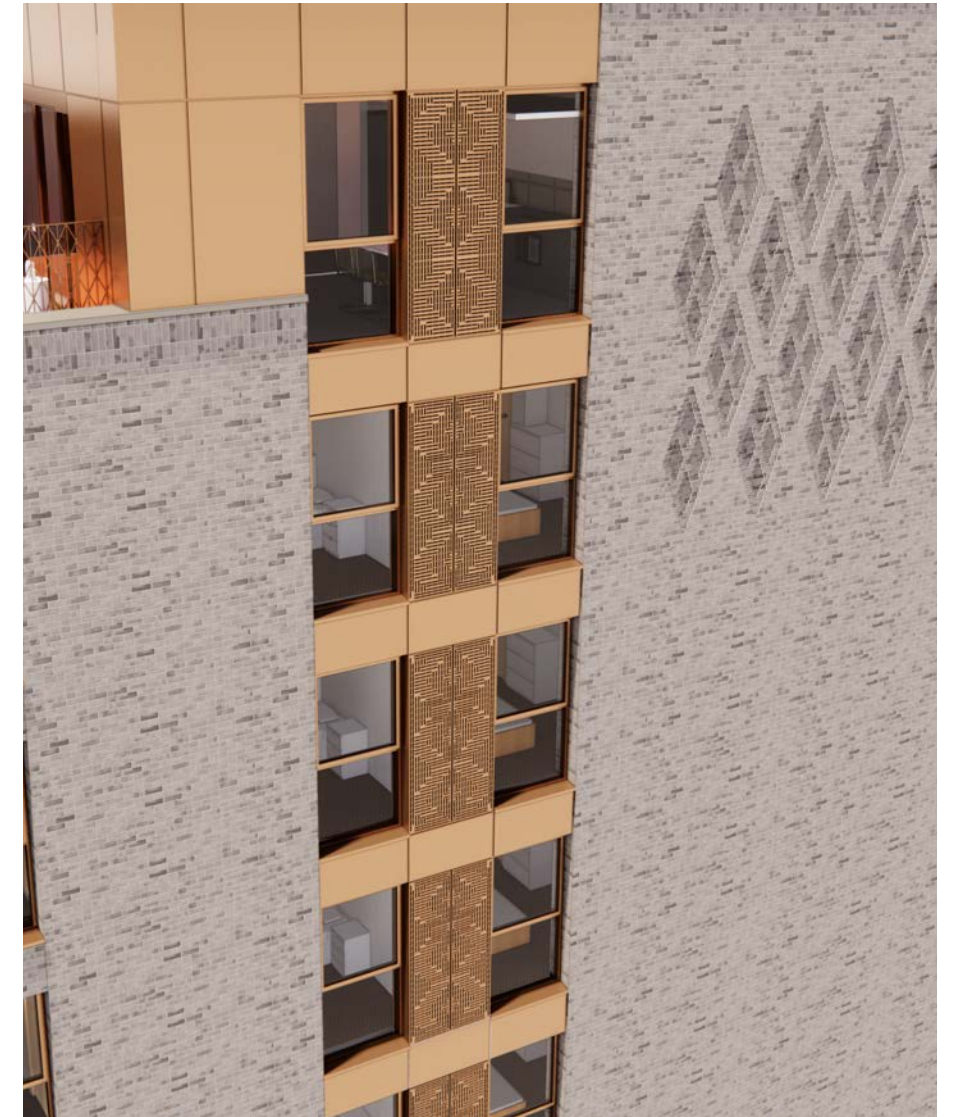
3D image of vertical perforated panels on south-west facade
