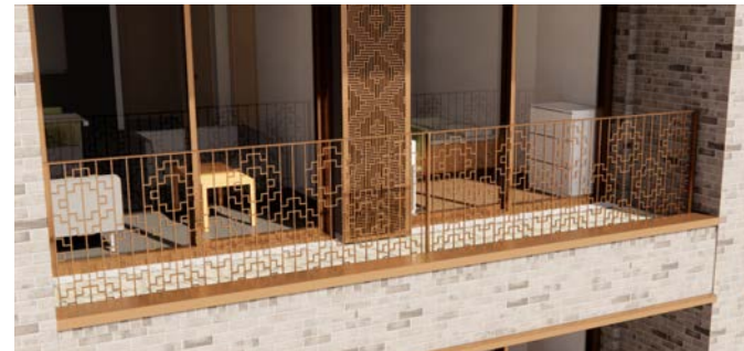
Option 04 Pros - closely aligns with 'textile' motif pattern, visual permeability, bespoke and decorative. Cons - pattern too similar to perforated panels, would need to be constructed as 'face-fixed' zig-zags rather than integral to the railing design.
