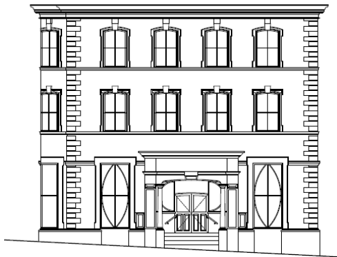
EXISTING NORTHWEST ELEVATION CLARENCE STREET FACADE
