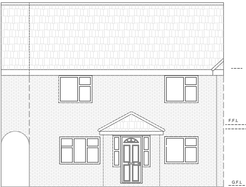
EXISTING FRONT ELEVATION
