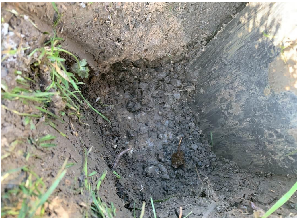
Soil Pit, western side of Pitch A – hard, impermeable and stony subsoil.
