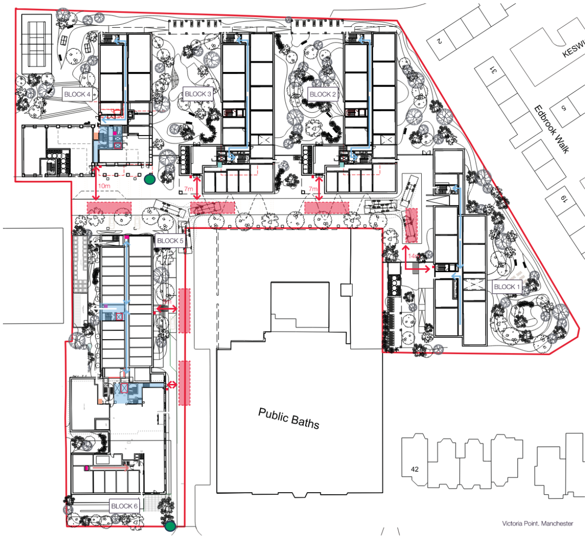
Figure 7: Fire Service Vehicle Access (Hydrants Marked in Green)
