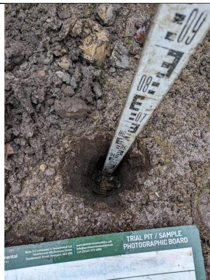
Hand dug pit HP1: Internal view of excavation
