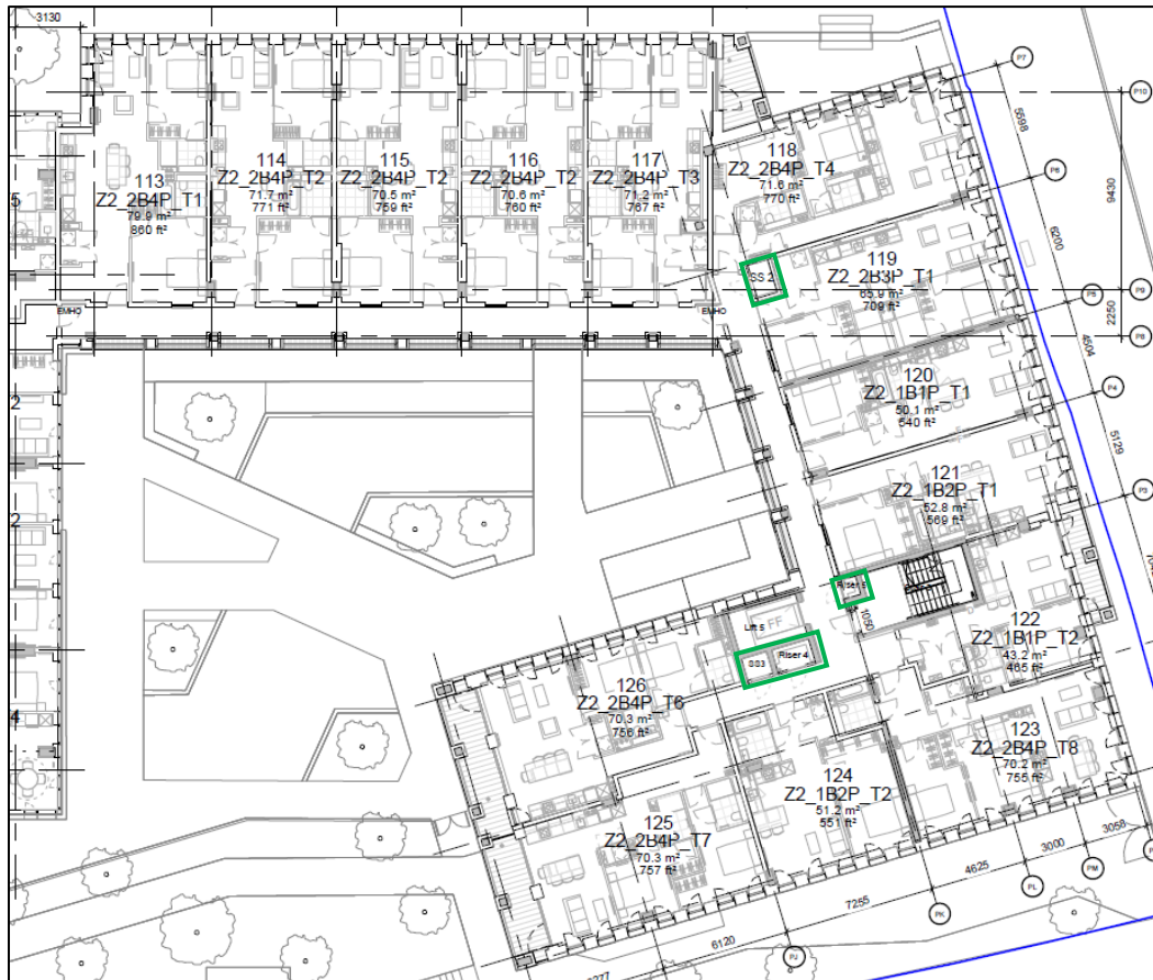
Figure 6: Location of service risers – Podium
