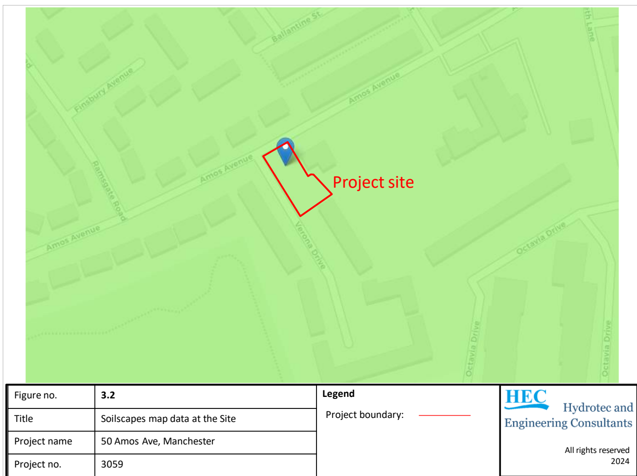
Figure 3.2: The soil types beneath the Site – slowly permeable, seasonally wet and acid-loamy and clayey soils (reference - Soilsclapes map data of Cranfield University 21 ).
