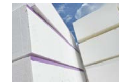
Expanded polystyrene (EPS) e.g. Filcor by Cordek - assumed @ 50kg/m3
