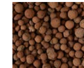
Lightweight expanded clay aggregate (LECA) - assumed @ 350kg/m3
