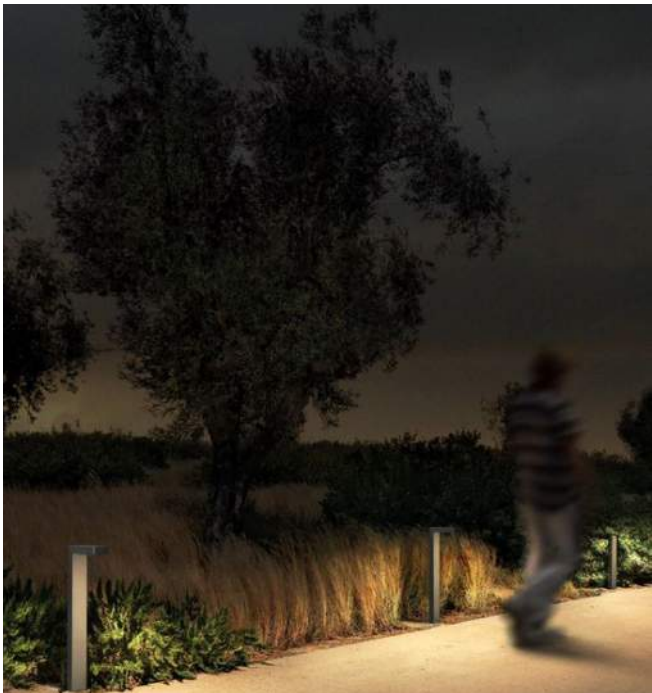
Figure 37: Directional lighting to avoid upward lighting
