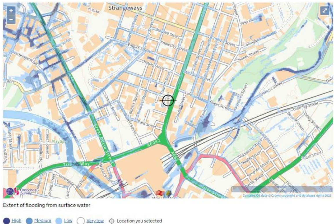
Figure 4.2: Risk of Flooding from Surface Water
