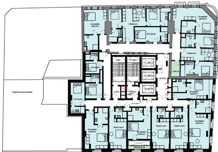
Figure 6. Level 2 Floor Plan (typical lower level hotel floor plan)
