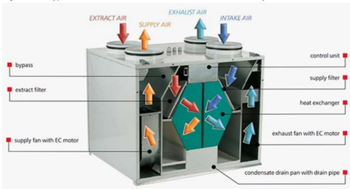
Figure 2: A typical residential mechanical ventilation with heat recovery unit
