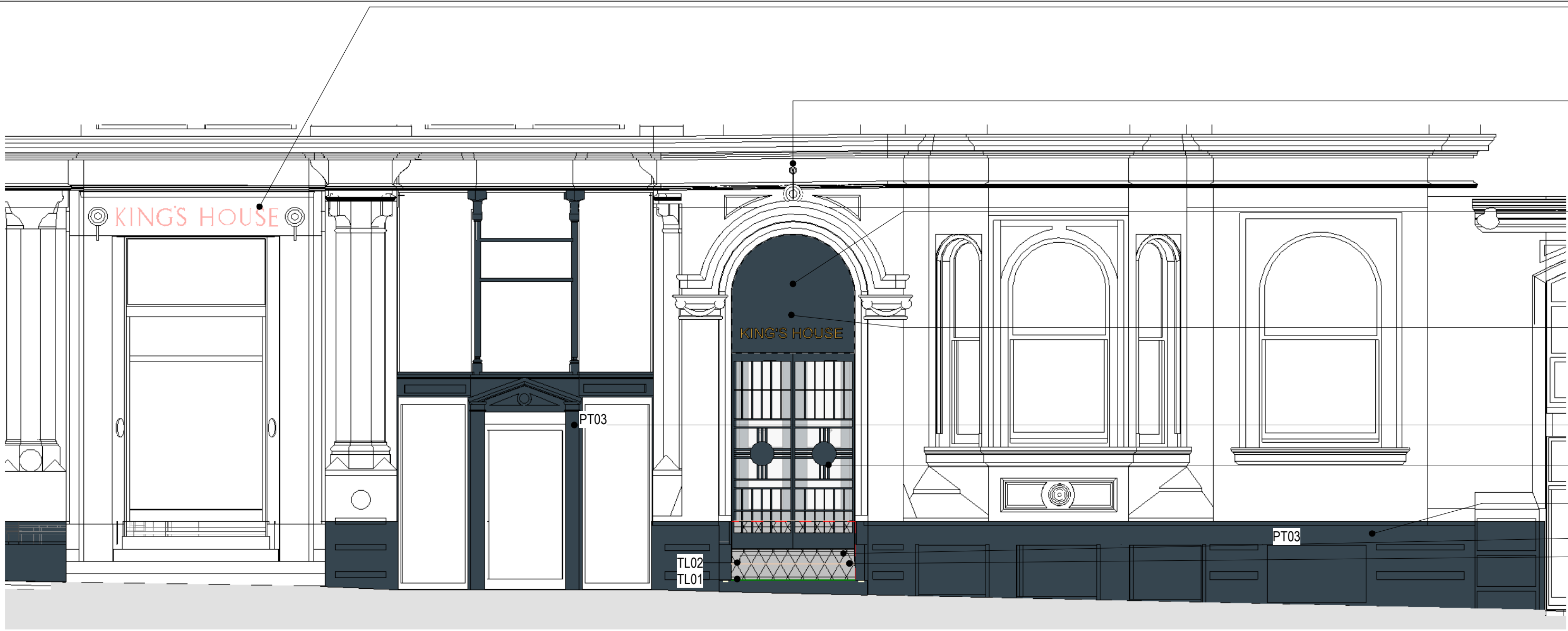
North Elevation External Glazing & Finishes 1 : 50
