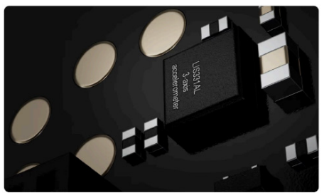
Built-in accelerometer: reports dismantling and impacts
