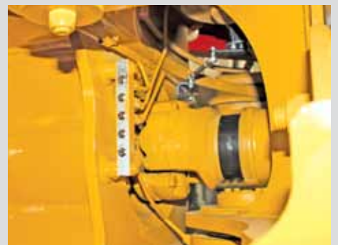
The centralised lube bank places difficult-to-reach nipples within reach. The convenient lube chart helps ensure that nothing gets overlooked.
