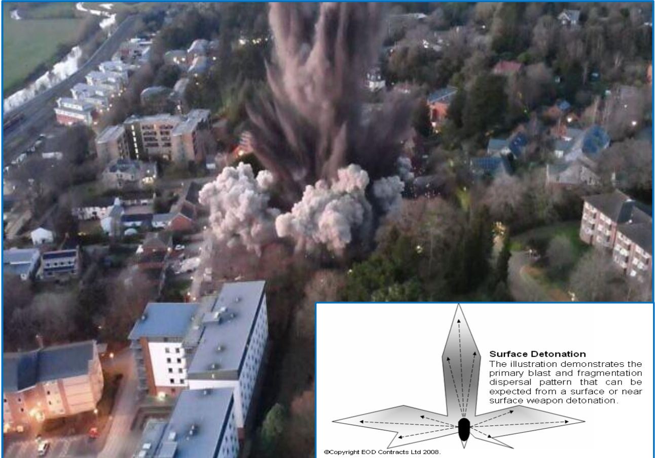
Figure 6.1: Primary Blast &amp; Fragmentation on Land
