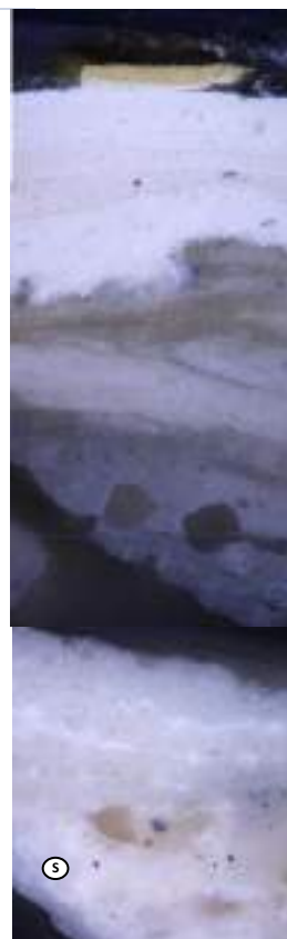
Sample 21AB (200x mag) – ceiling, moulding to edge of ceiling panel.
