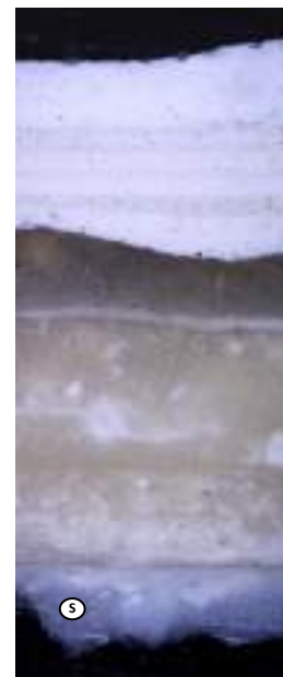
Sample 26 (200x mag) – ceiling, beam casing, large flat (middle area)
