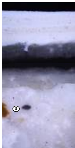
Sample 20 (200x mag) – ceiling, flat panel (behind later plasterboard)
