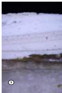
Sample 25 (200x mag) – ceiling, beam casing, ovolo moulding
