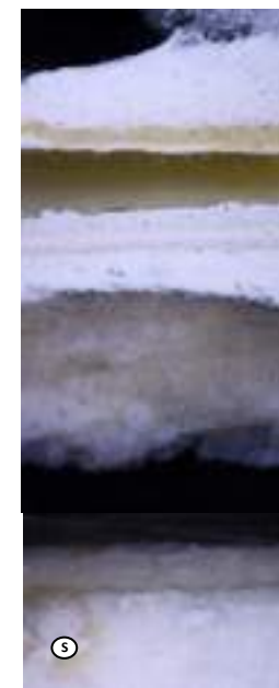
Sample 22 (200x mag) - ceiling, outer moulding – outside of gypsum skim.
