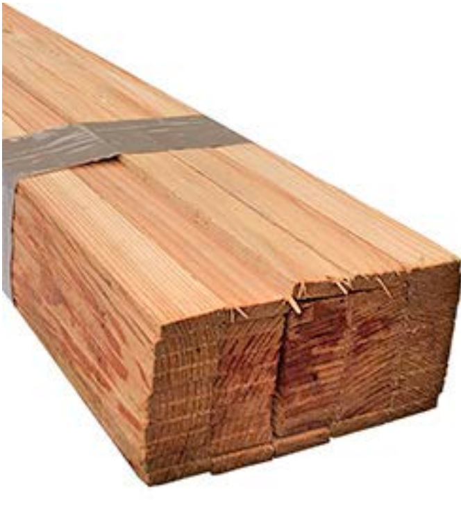
313 Timber laths Supplier: CONSERV, Lee Road, Bolckow Industrial Estate, Middlesbrough TS6 7AR, 01642430099, support@conserv.co.uk (or similar and approved). Material: Larch ( Larix decidua ) / Sweet chestnut ( Castanea sativa ). Type: Sawn (larch) / Riven (sweet chestnut). Cross sectional size: 26mm x 6mm (larch) / 32mm x 6mm (sweet chestnut) Length: 1.22m (larch) Spacing: Typically 10mm between laths, no less than twice the largest aggregate size. Joints: Lath trimmed at end to finish on a joist. Nom. 3mm space to allow for expansion. Joints staggered every 12 laths. Fixing: Stainless steel ring shank nails, min 40mm in length. Installation: Fully immersed in water for min. 7 days prior to fixing.
