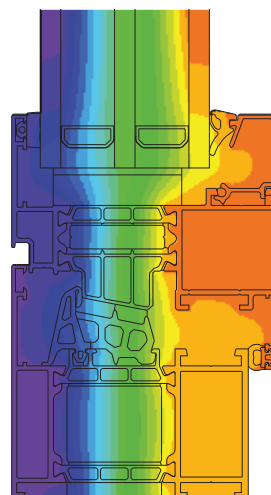
Distribution of isotherms in MB-79N SI window
