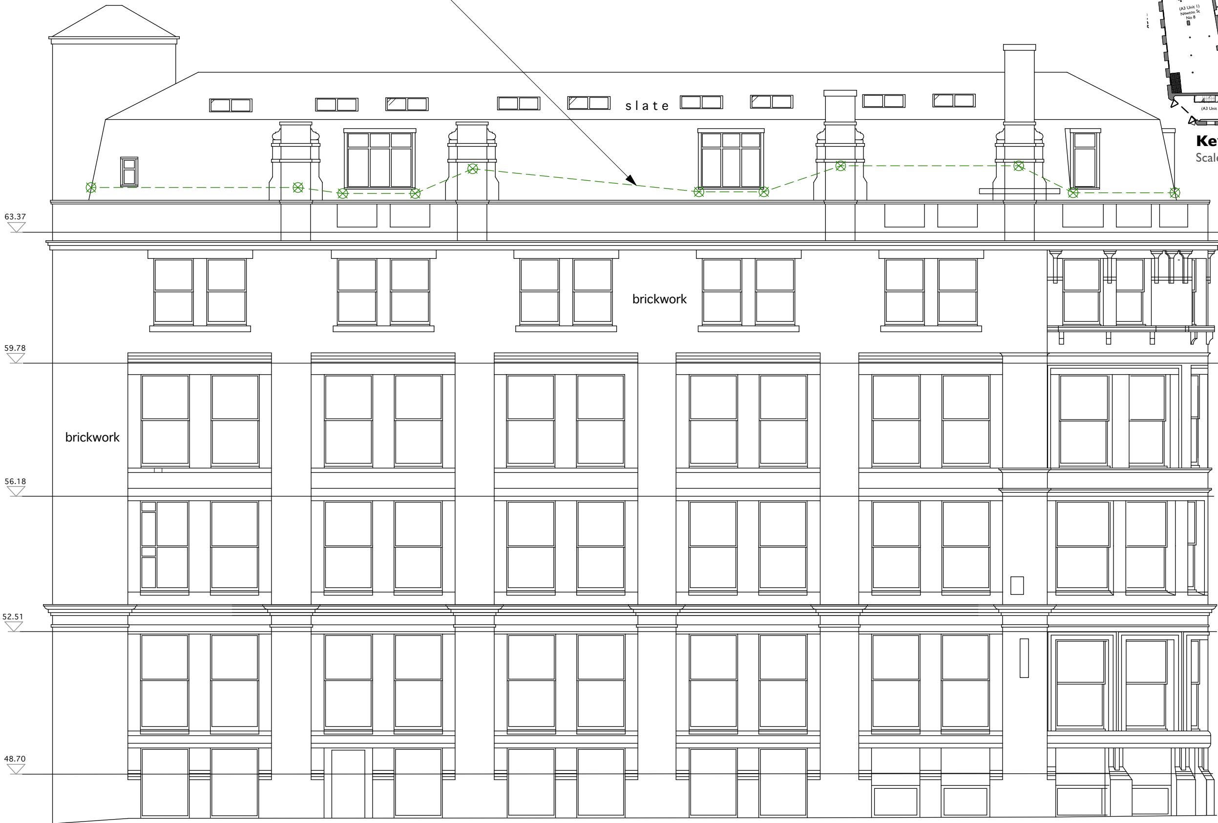
Proposed Elevation - Dale Street Scale 1:100
