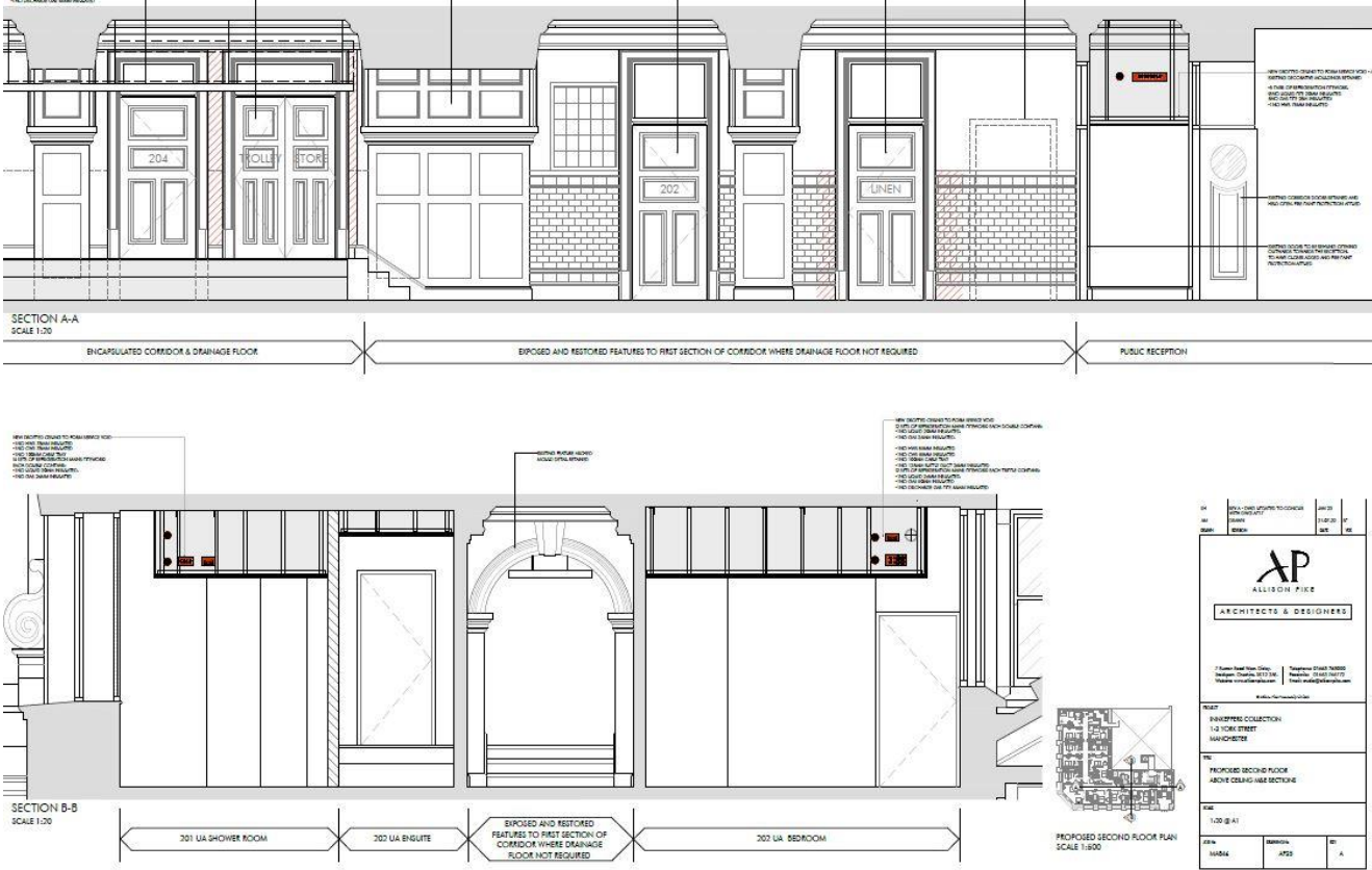
Fig 6: Area at second floor (shown grey on plan) where there are no original corridor features remaining – this has been opened-out in the 1980s with a concrete or steel frame structure inserted in the space – proposed to have a fully enclosed ceiling.
