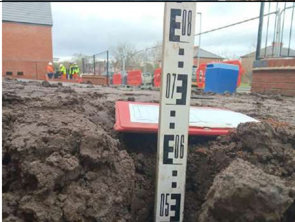
Photograph 3 Evidence of suitably chemically validated topsoil with a minimum of 150mm growing medium in shared front garden areas (Plots 7-8) over natural strata.
