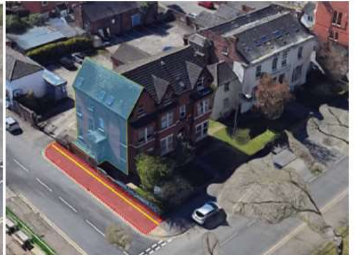
Protection scaffold (Blue) footpath encroachment (Yellow)
