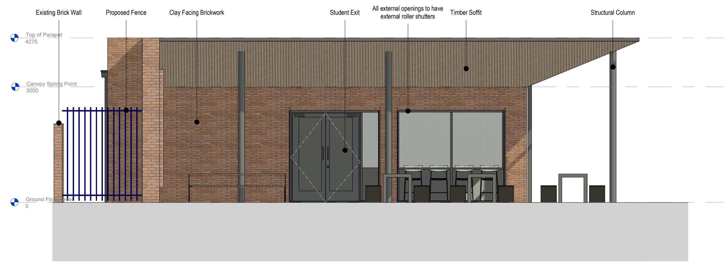
3 South Side Elevation 1: 50 Ref Sheet: 0711
