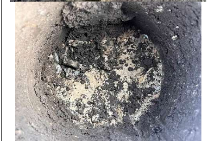
Photograph 17: Evidence of suitably chemically validated topsoil with a minimum of 150mm growing medium in garden areas (Plot 12).
