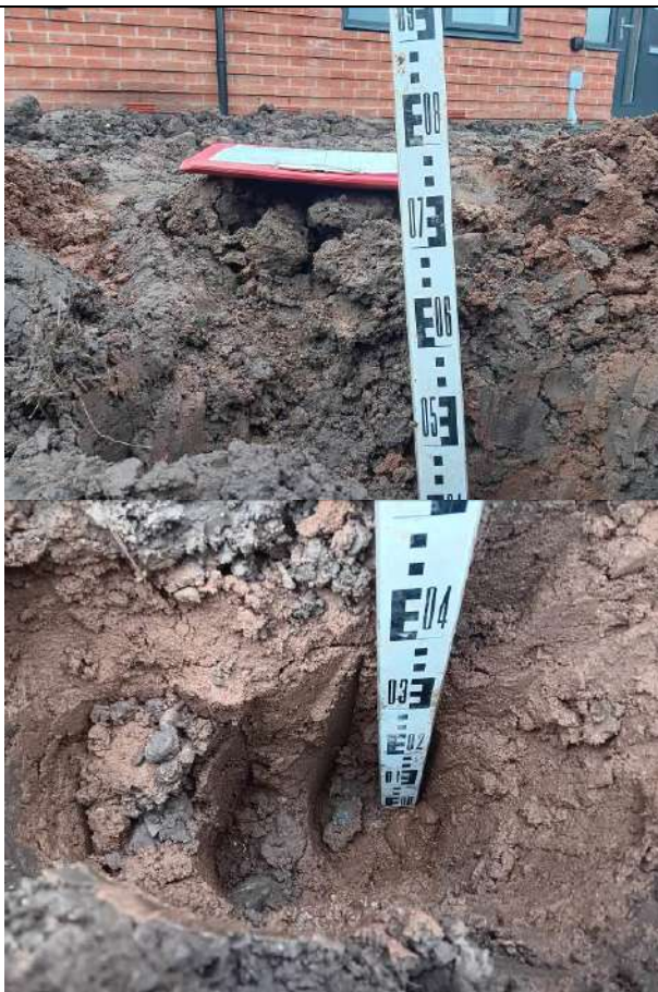
Photograph 5: Evidence of suitably chemically validated topsoil with a minimum of 150mm growing medium in shared front garden areas (Plots 9-10).
