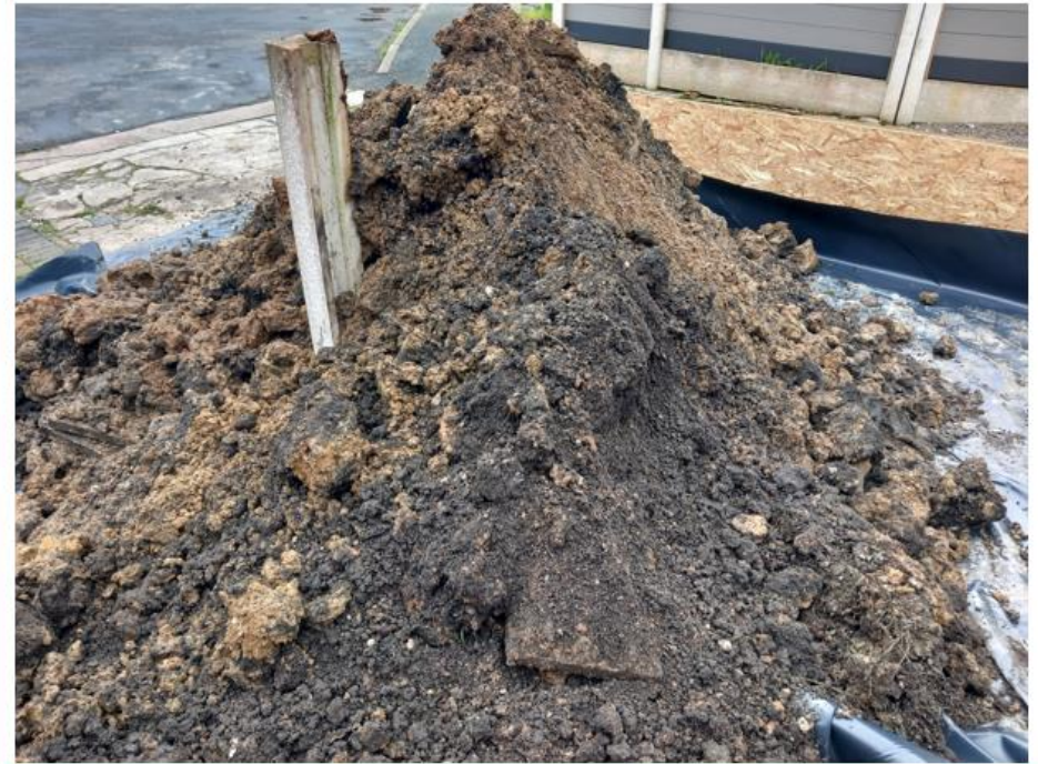
Photo No.12: Arisings heap ready for removal offsite showing relict topsoil material and natural, sandy Clays
