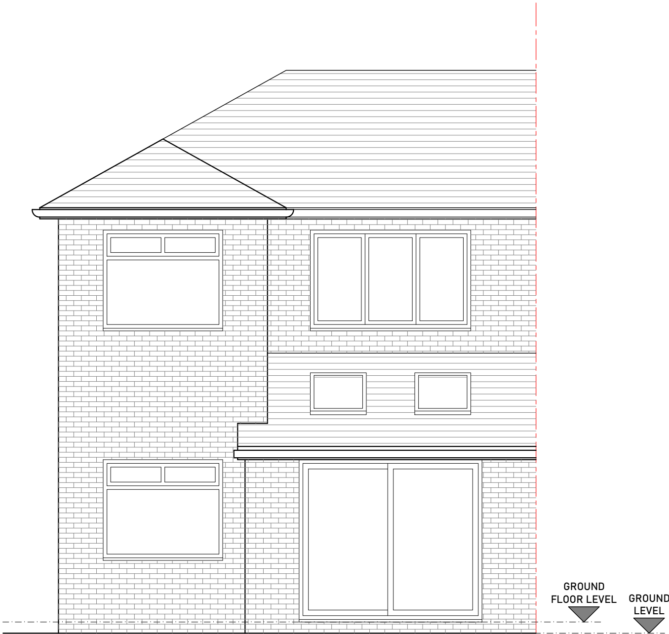
EXISTING REAR ELEVATION 1:50
