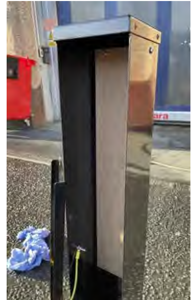
Figure 3 – An R150 after IPX4 test performed at Ritherdon
