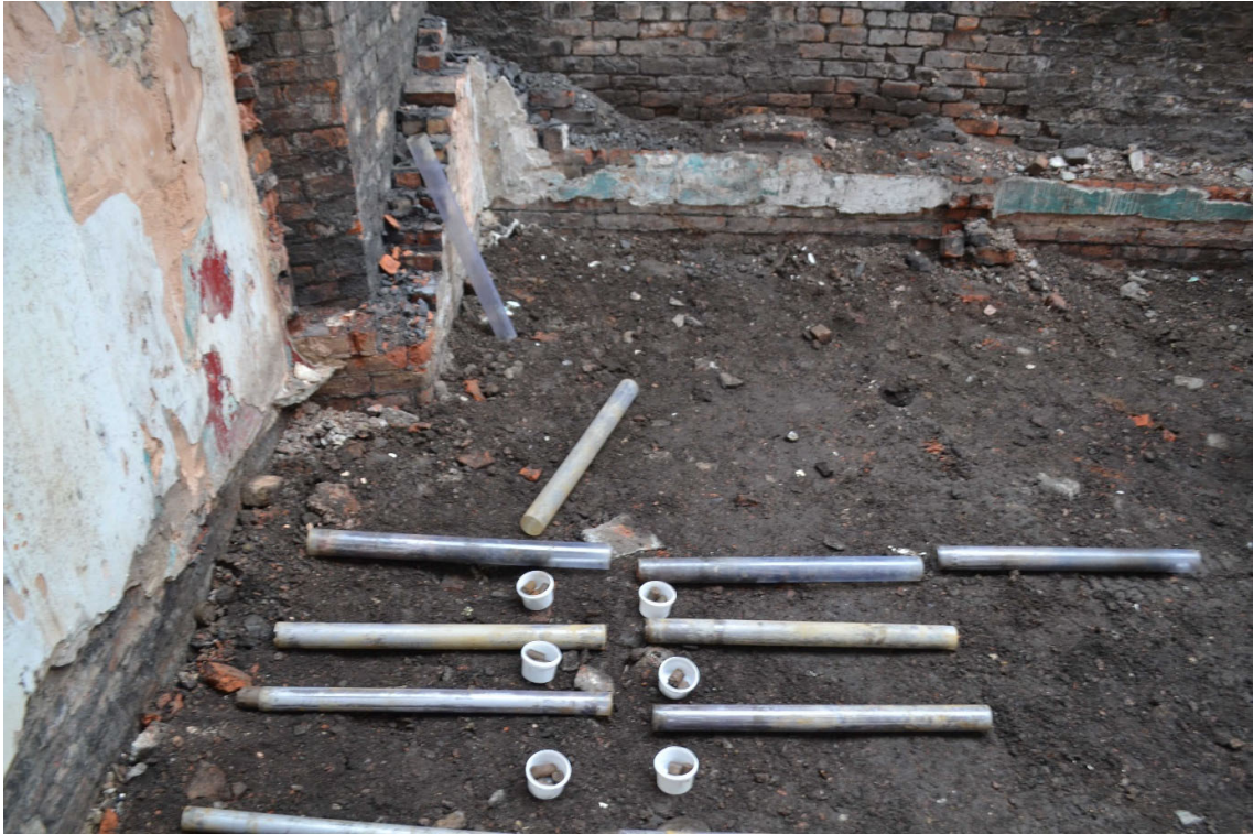
Plate 3: Arisings from Borehole 2
