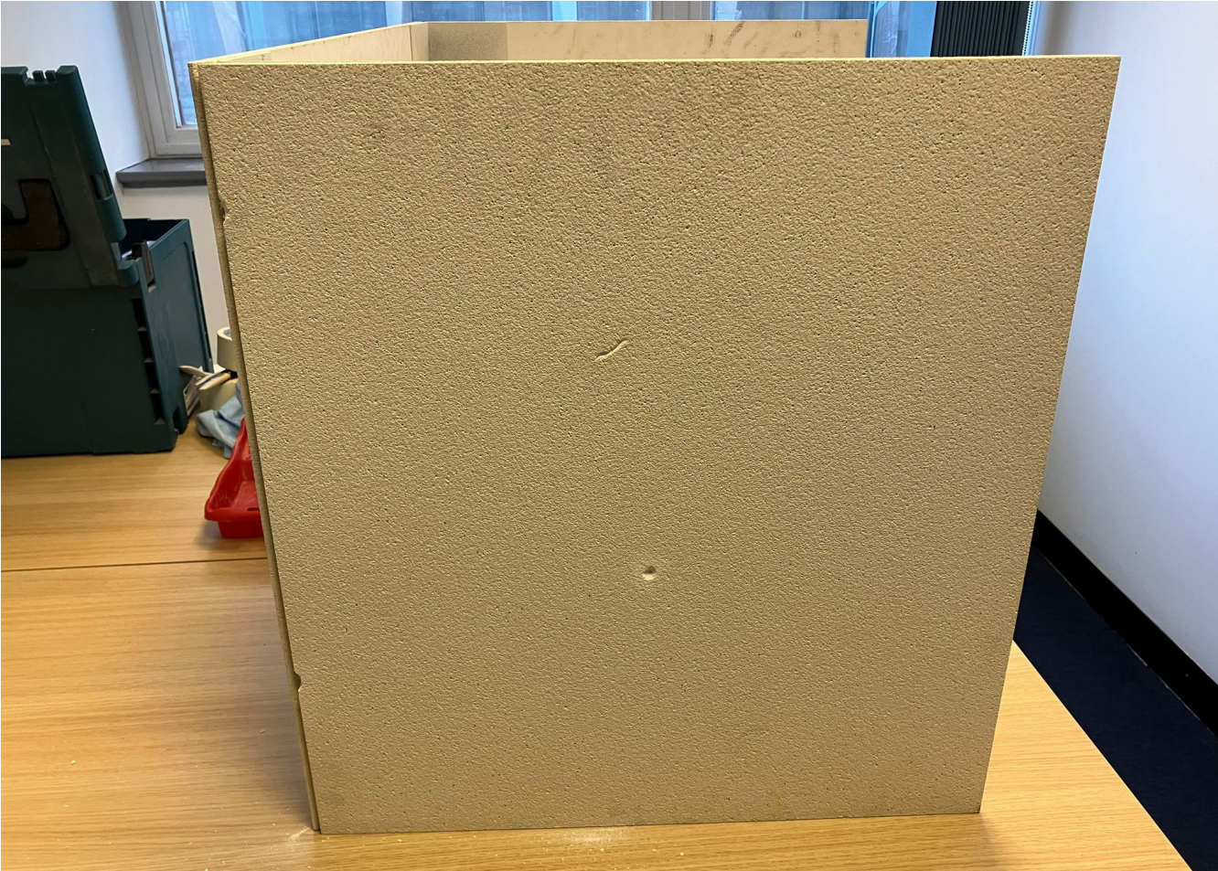
GRC sample damaged
