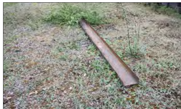
Channel section beam on the deck of the viaduct
