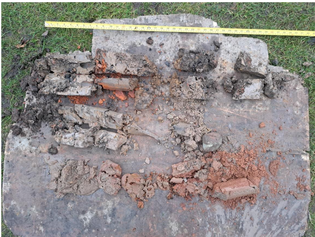
Photograph 12 WS02 drilling arisings (top to bottom, left to right).
