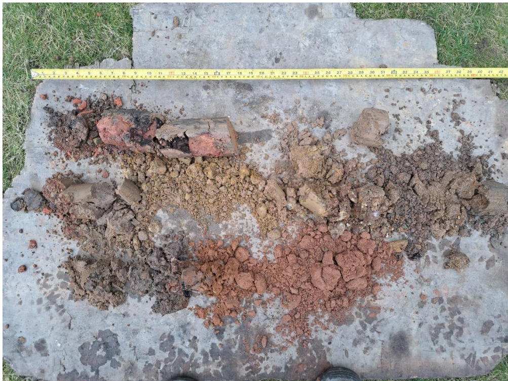
Photograph 10 WS05 drilling arisings (top to bottom, left to right).
