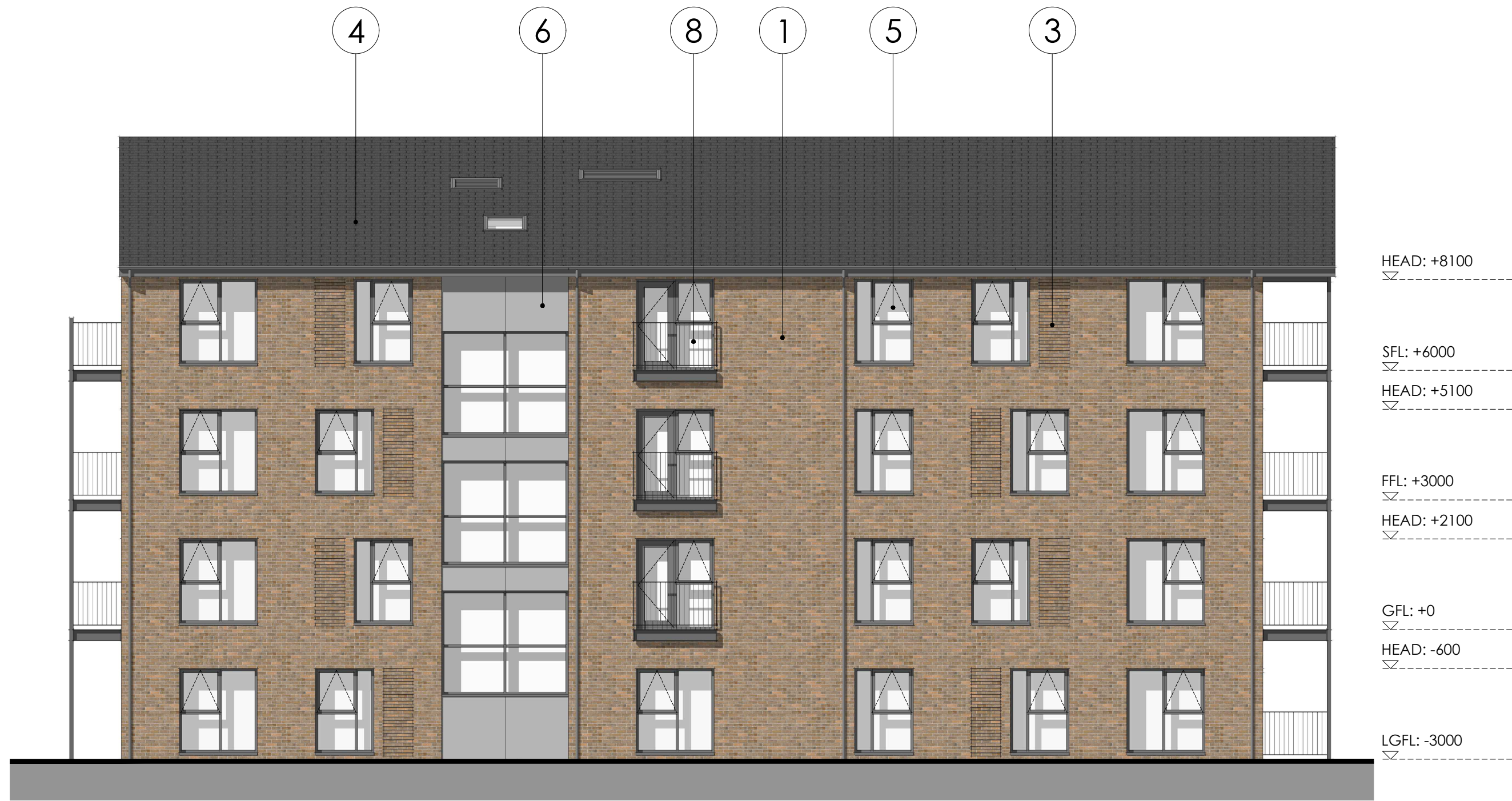
Apartment Block Delaunays Road Elevation A 1:100
