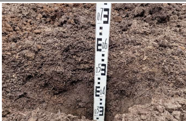
Close view of Staff - Total 600mm depth achieved.
