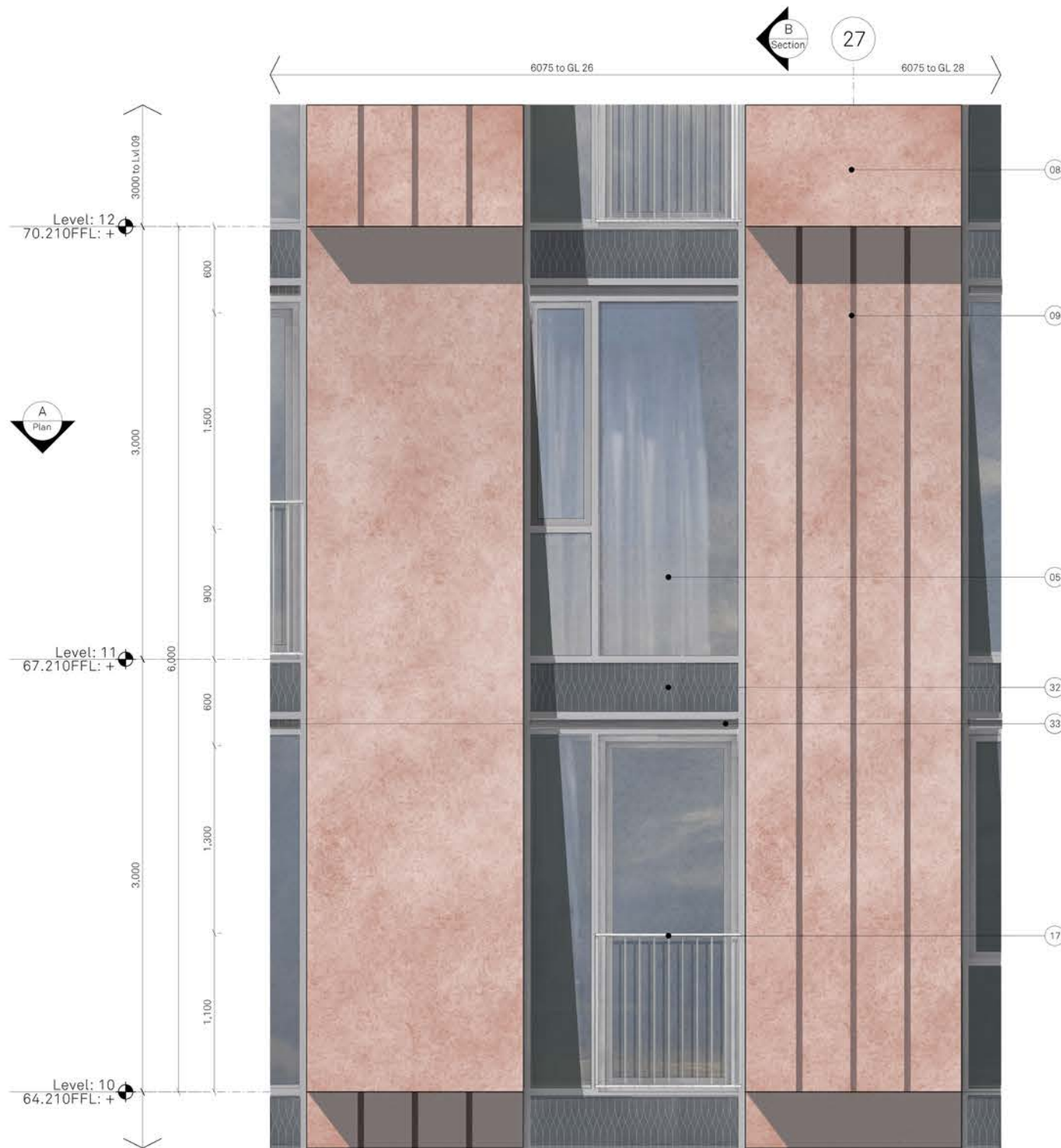
ELEVATION A Typical Bay
