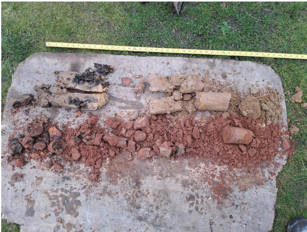
Photograph 6 WS03 drilling arisings (top to bottom, left to right).
