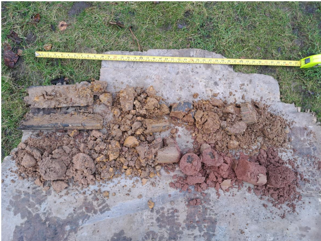
Photograph 2 WS01 drilling arisings (top to bottom, left to right) .
