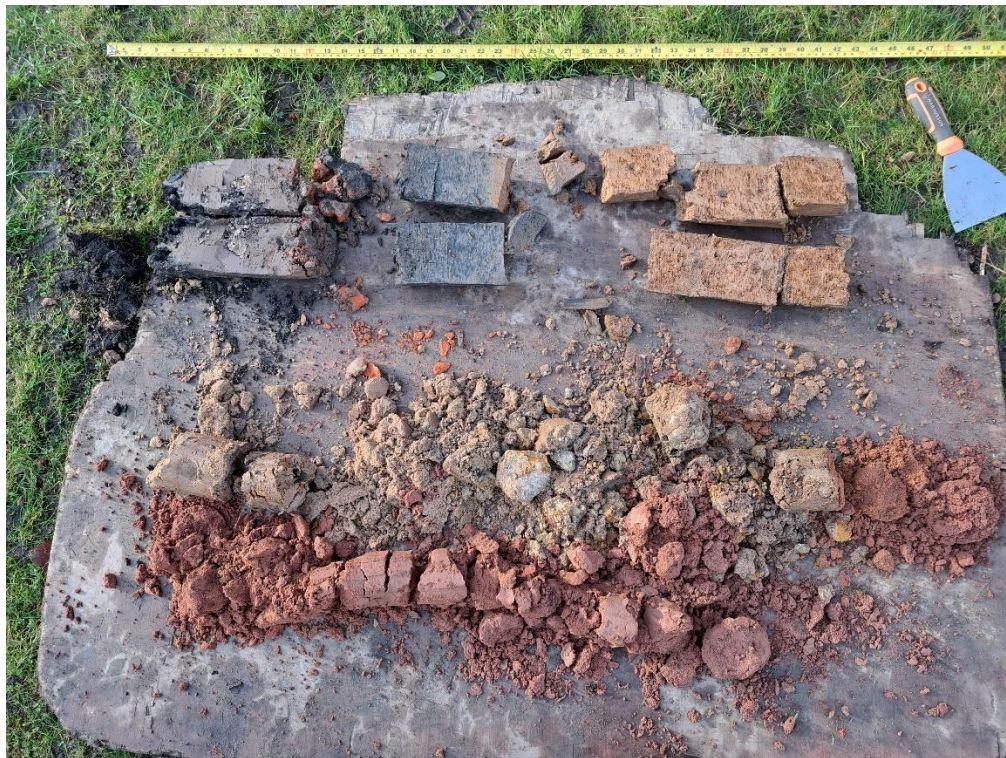
Photograph 4 WS02 drilling arisings (top to bottom, left to right).
