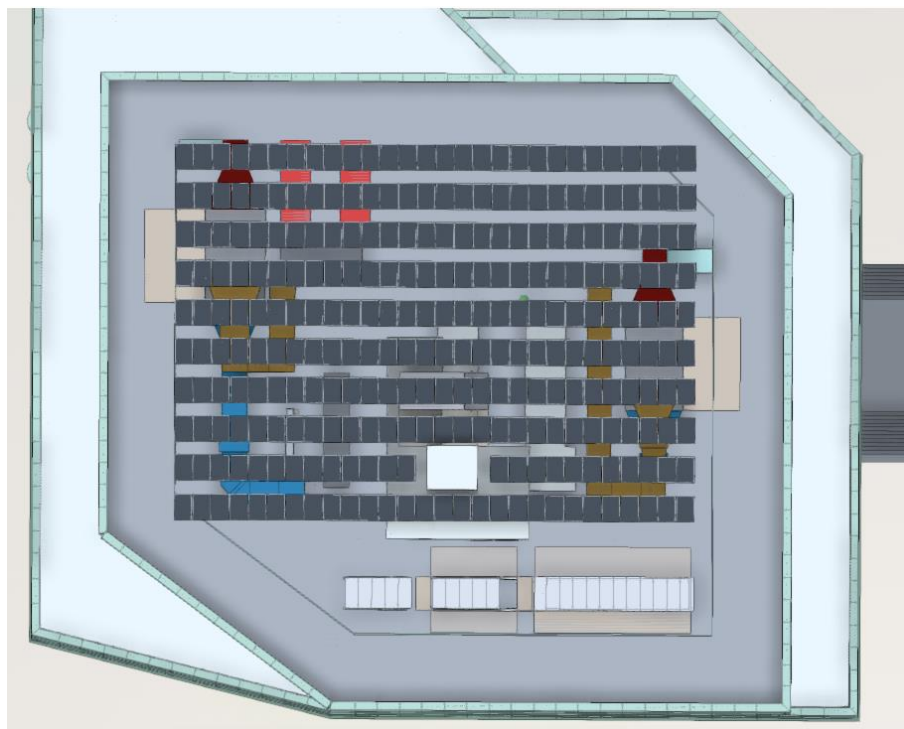
Figure 5-1 - PV location on the roof
